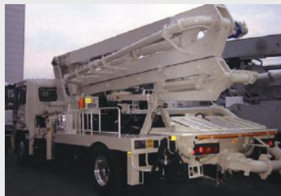
Concrete Pump Truck
